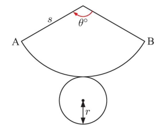
For the net of a cone alongside, notice that the length of arc AB must equal the circumference of the base circle.
