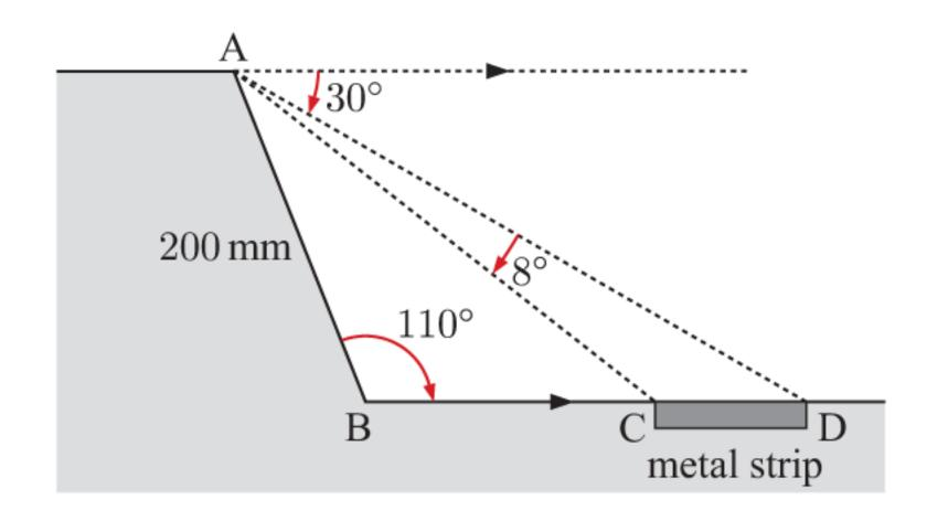
The cross-section design of the kerbing for a driverless-bus roadway is shown opposite. The metal strip is inlaid into the concrete and is used to control the direction and speed of the bus. Find the width of the metal strip.
