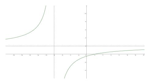
The graph has a vertical asymptote x = -8, horizontal asymptote y = 2 and x-intercept at x = 2.
