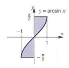
Sketch the graph to find the end points; since the volume of revolution is about the *y*-axis, *y* limits will be required.
