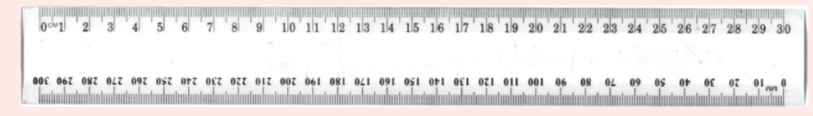
A ruler measures length. In the Metric System it measures in centimetres and millimetres, and can measure to the nearest millimetre. Its accuracy is  $\pm \frac{1}{2}$  mm.
