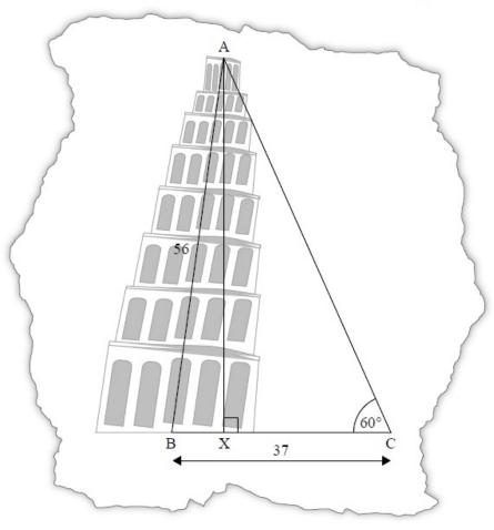
10a. Use Giovanni's diagram to show that angle ABC, the angle at which the [5 marks] Tower is leaning relative to the horizontal, is 85° to the nearest degree.
