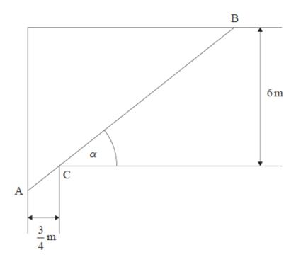
A narrow passageway with  $\frac{3}{4}$  m width is perpendicular to a room of width 6 m. There is a corner at point C. Points A and B are variable points on the base of the walls such that A, C and B lie on a straight line.
